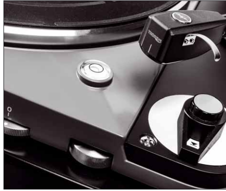
The knob on the right controls the electric tonearm lift. At the bottom center of the picture, you can see one of the knurled wheels for height adjustment
