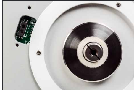
On the left, the reflex light barrier that determines the platter speed
