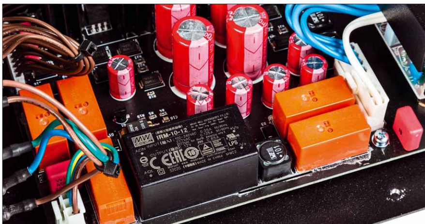
A second switching power supply keeps parts of the digital technology „alive“ in standby mode
