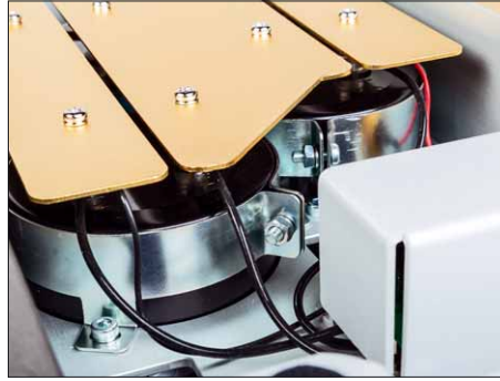
The supply concept of the Grand Master electronics relies on huge amounts of screening capacity
