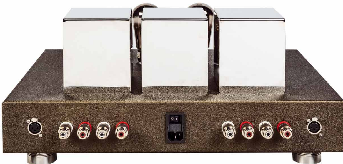
The two speaker outputs are separate 16-ohm transformer windings and are typically operated in parallel
