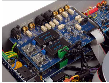
The preamplifier section with the partially encapsulated modules sits directly at the inputs. Signal processing is exclusively symmetrical from here on. On the right is the phono board
