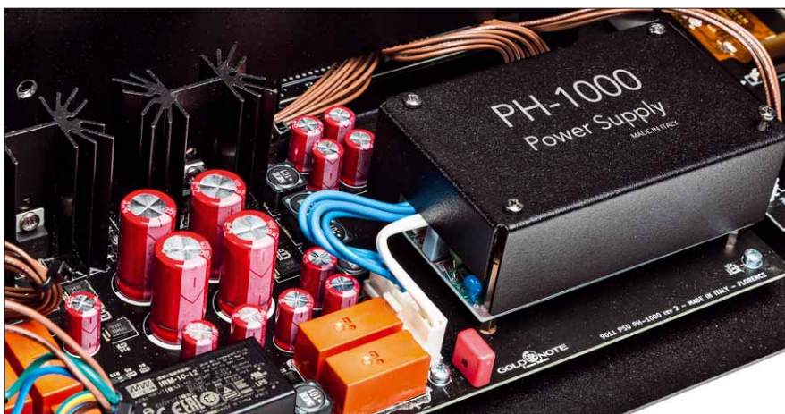
A switching power supply sits under the metal lid of the power supply
