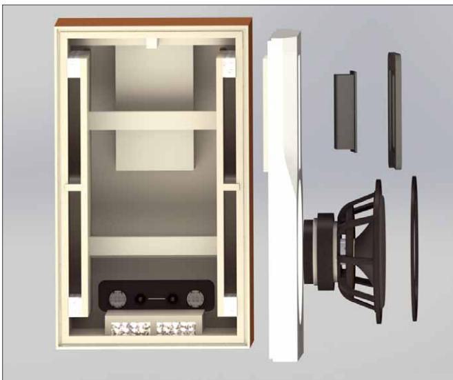
The cabinet is an elaborate affair with a multitude of struts and resonance chambers
