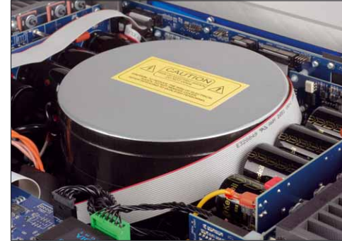
The mighty toroidal transformer is specified with 1,000 watts and thus defines the ample power reserves of the FLS9
