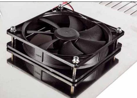
The fan is indispensable due to the heat dissipation of the device but inaudible
