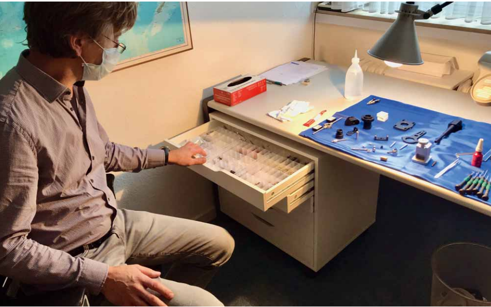
Thomas Pütz, newly hired only for the production of this tonearm, at his workstation where he is assembling the bearings for the next batch
