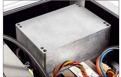
Effective sound insulation: This box contains part of the air supply system
