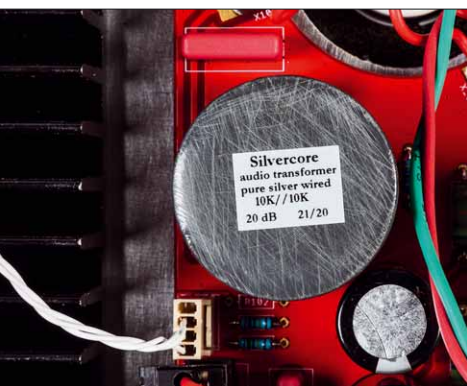
The silver input transformer also allows genuine symmetrical connection
