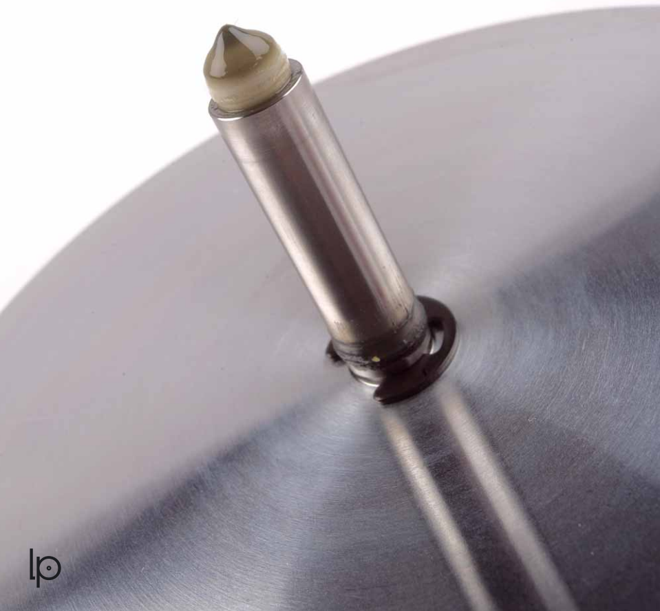
The platter axle with ceramic ball for the vertical forces
