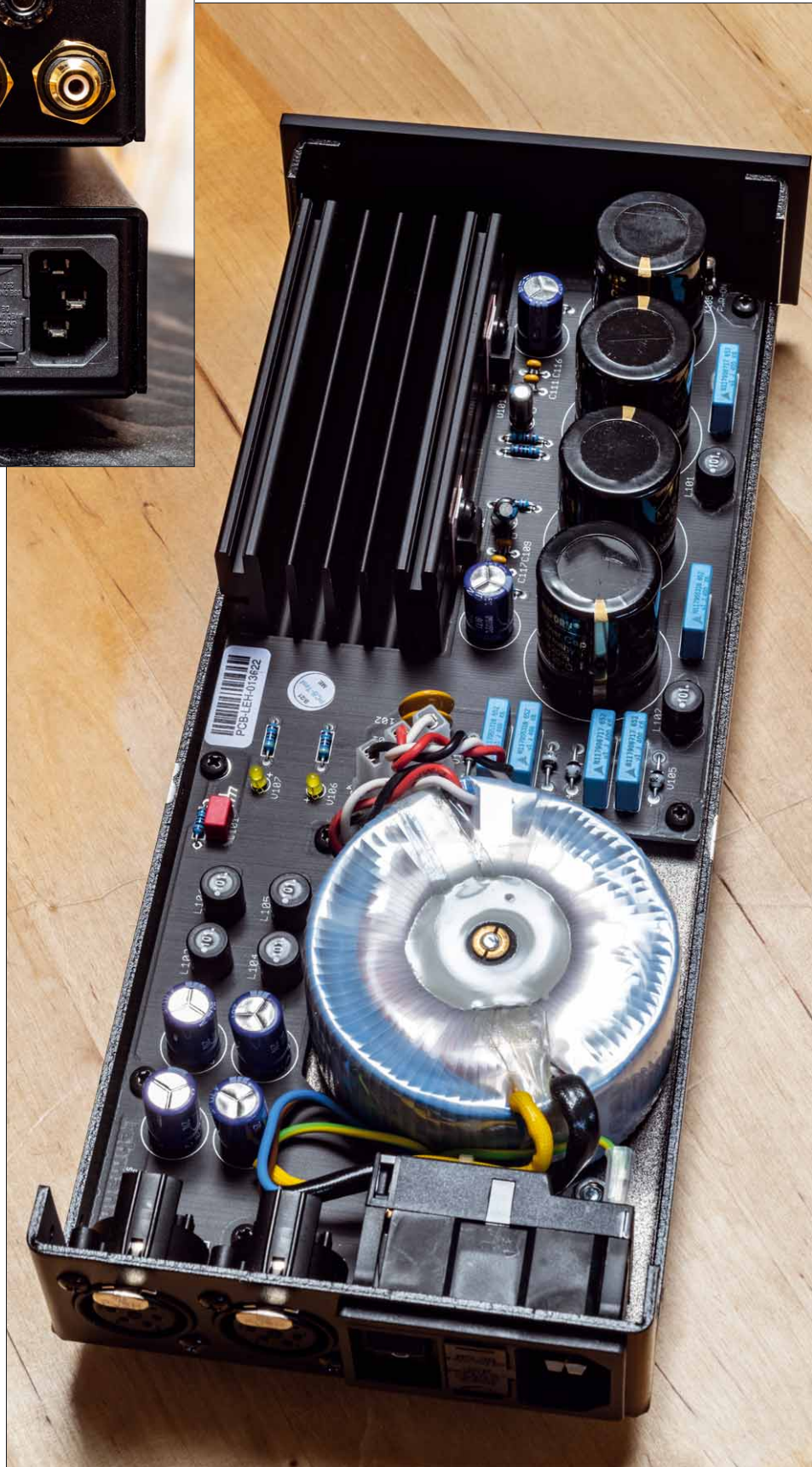
The power supply with toroidal transformer, ample filtering, and voltage regulation
