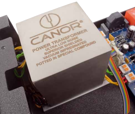
The transformer labors under a shielding hood
