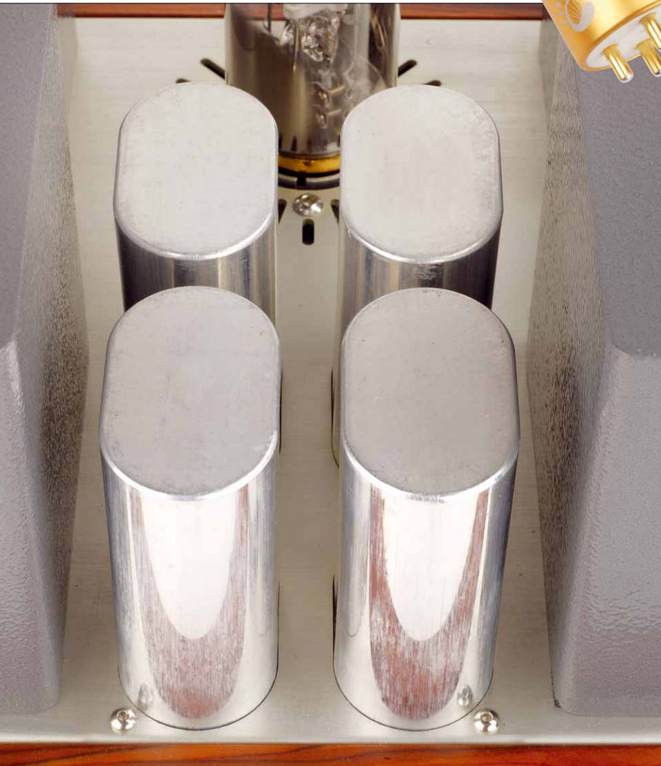
Large oil paper capacitors sift the high voltage
