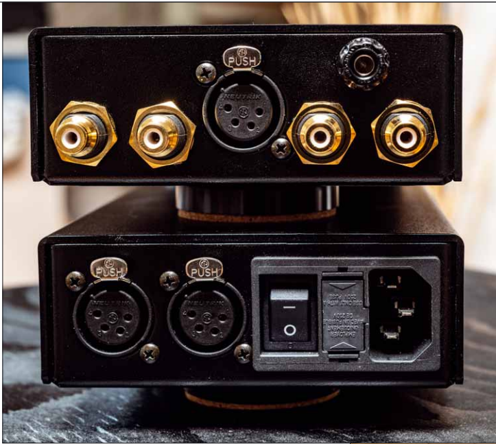
The small back panels of the device are entirely occupied with connectors
