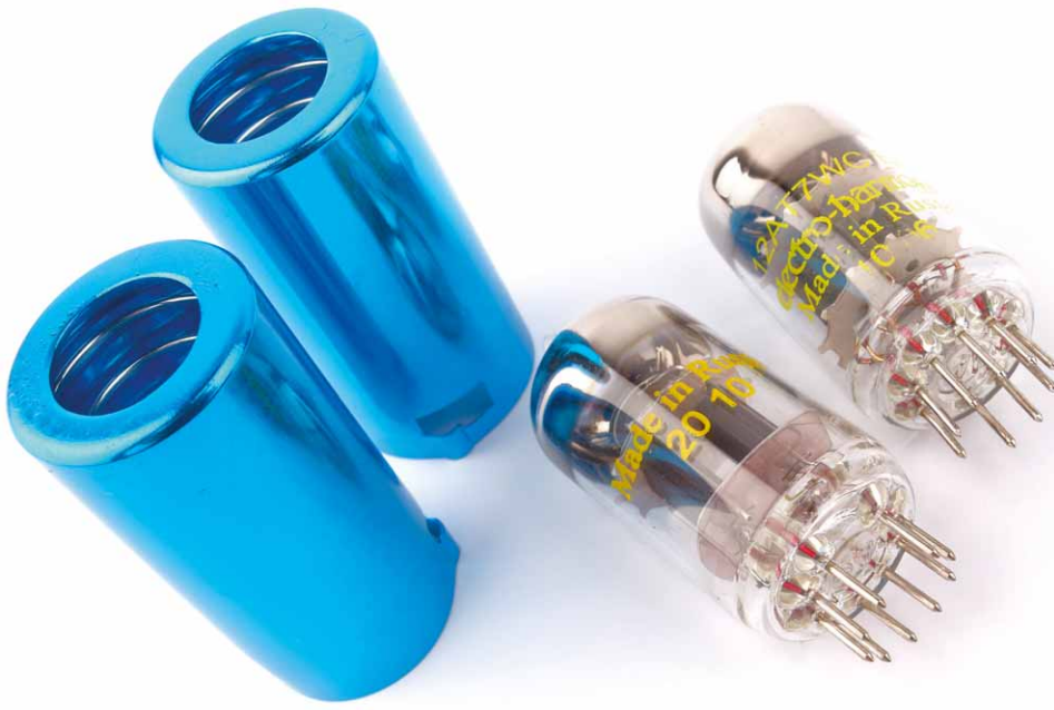
Under the shielding cap are double triodes from Electro Harmonix
