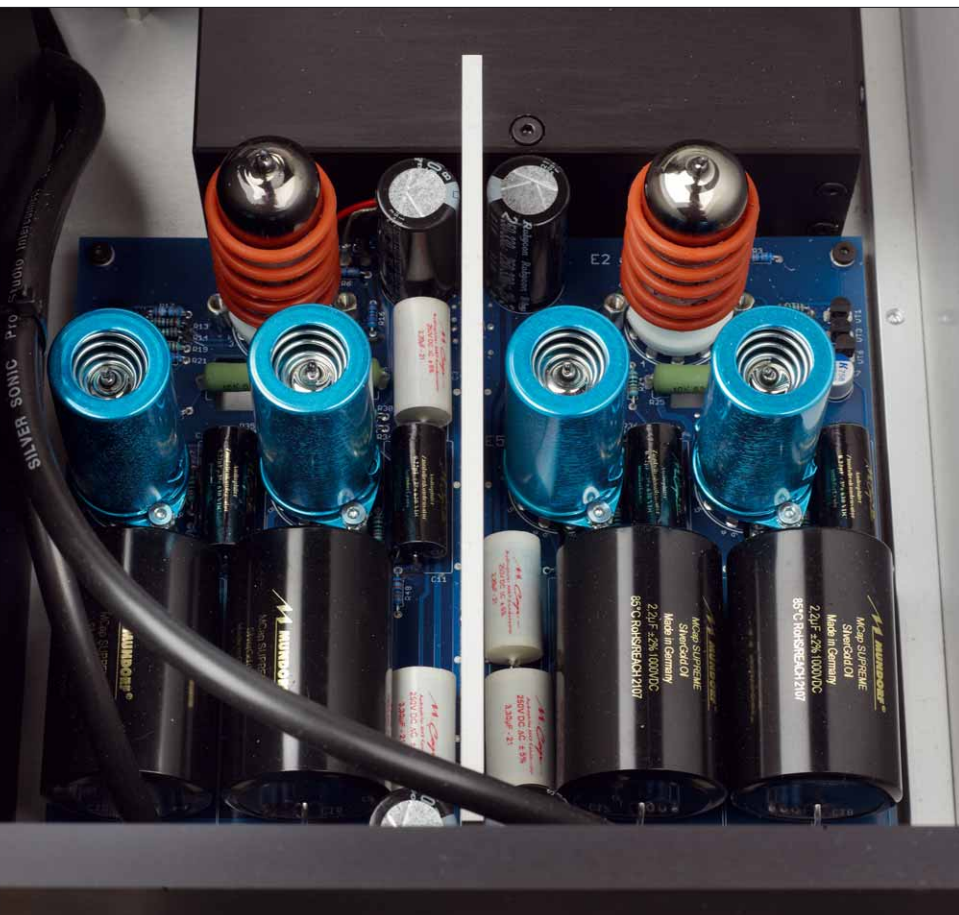
The preamp's symmetrical amplifier circuitry is impressively short
