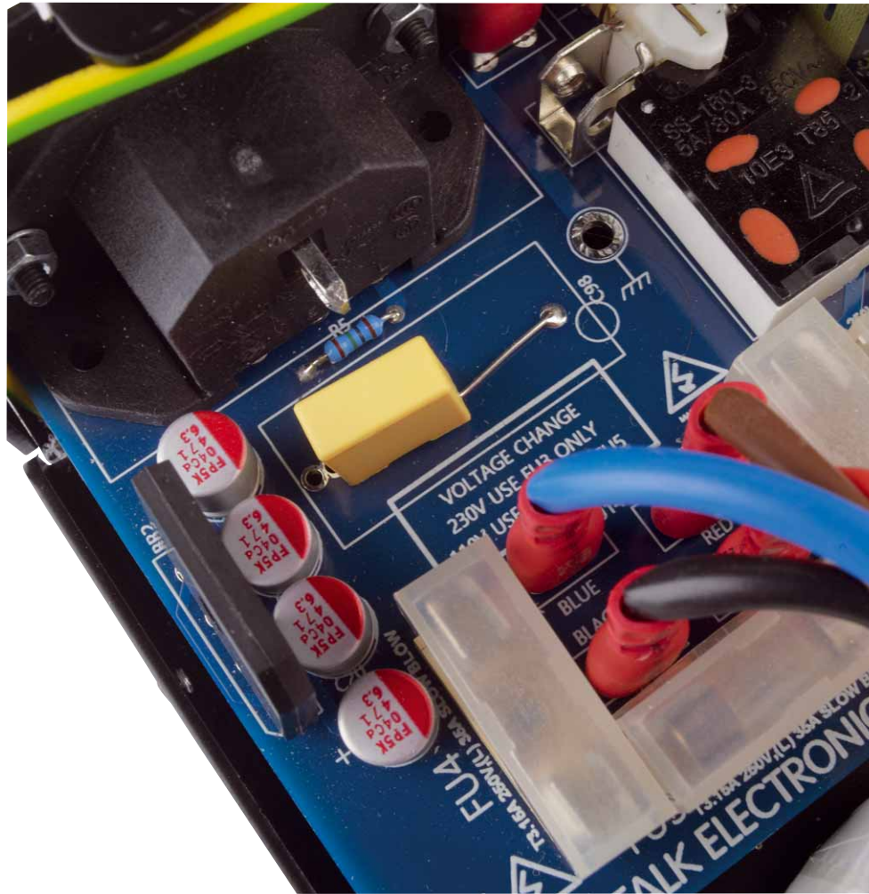
The developers even gave the device a DC filter at the mains input
