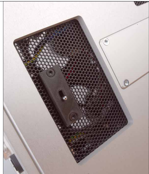
The switch for the negative feedback is well hidden at the bottom of the device
