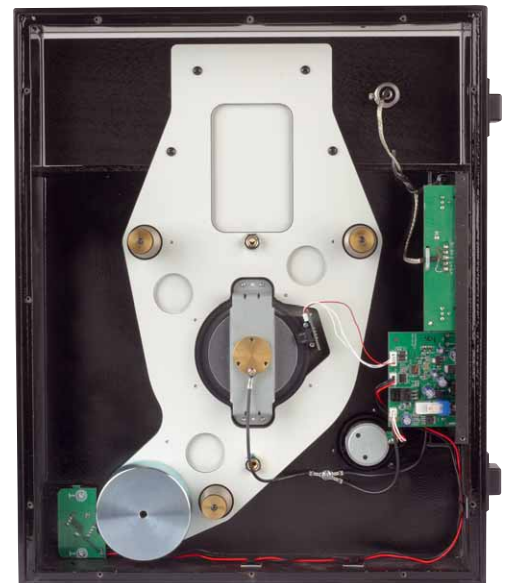
The beautifully simple TP 150 guides the cartridge on a J-shaped aluminum tube
