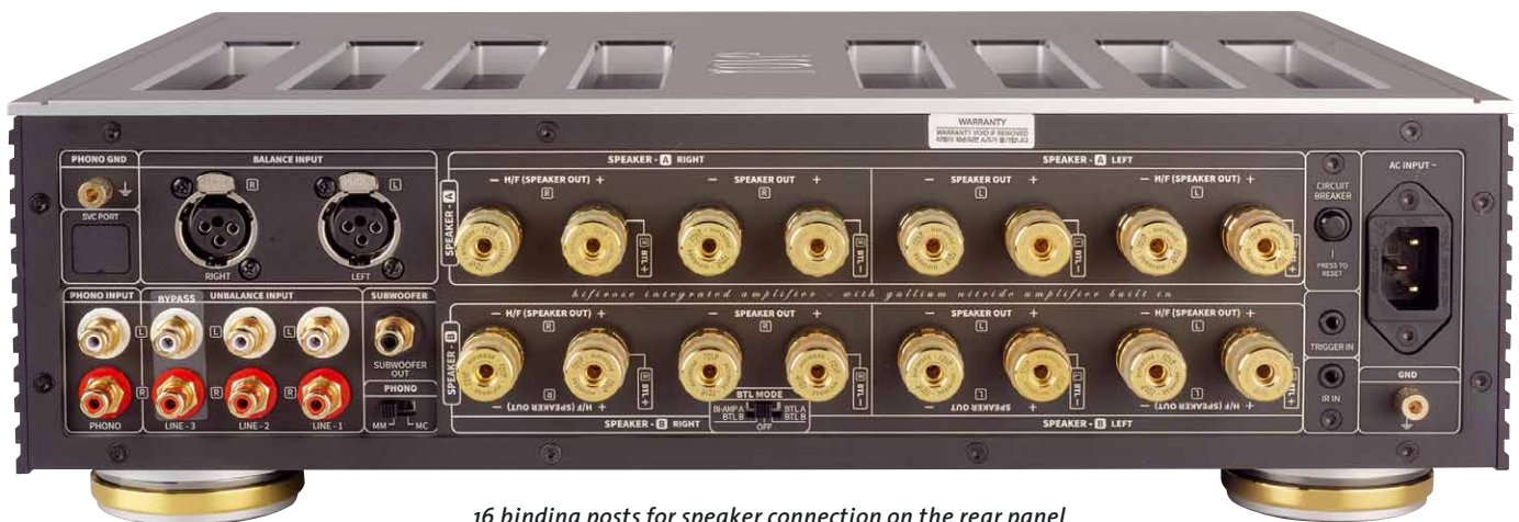
16 binding posts for speaker connection on the rear panel
