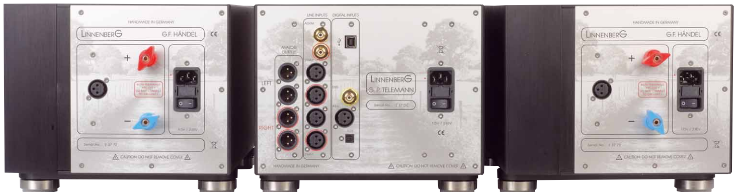
The power amplifiers are equipped with XLR inputs only. The preamplifier still has RCA connectors
