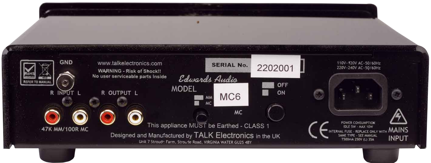
The power switch and MM/MC switch are on the back. Not optimal, but tolerable
