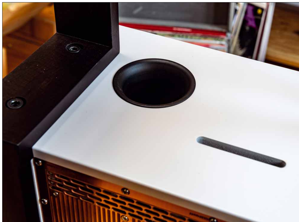
The offset reflex tube is tuned away from the textbook opinion
