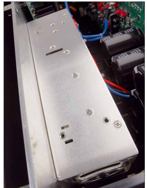
A pleasantly lightweight replacement for a bulky toroidal transformer is this switching power supply in the power stage
