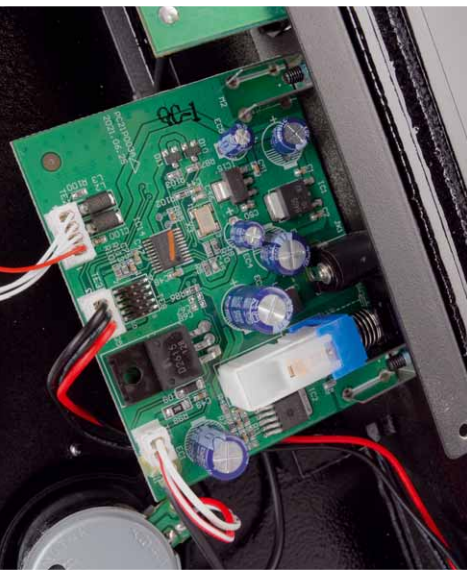
This is the motor controller board. It always ensures the correct speed with the help of the pulses from the speed sensor
