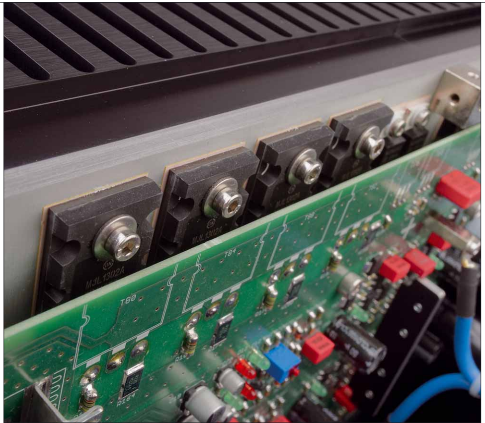
This is a quarter of the power amp transistors of a monoblock
