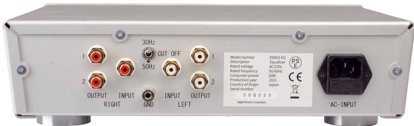
The back of the equalizer. One output runs through a subsonic filter; one doesn't
