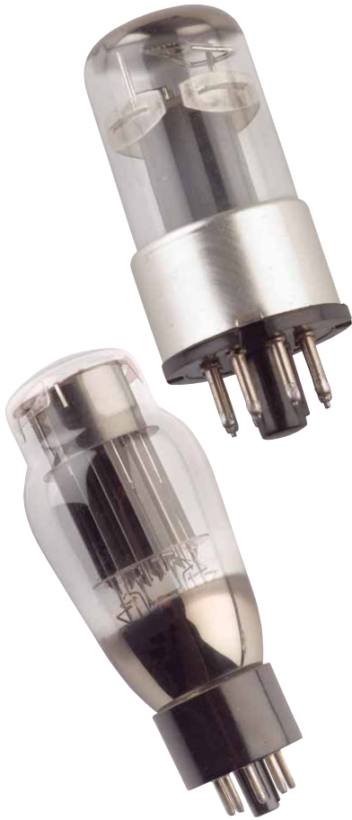
One 6AS7G per channel (left) acts as a driver for the large power tubes; a 6SN7 (above) provides part of the voltage amplification
