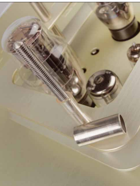
Pieces of tubing calm the individual layers of the „sheet metal“ towers
