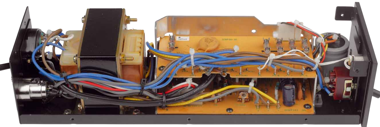
Built half a century ago, yet brand new: the power supply of the SP-10 MK2
