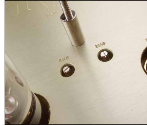
The quiescent current of the power amplifiers is adjusted with two potentiometers on the driver block
