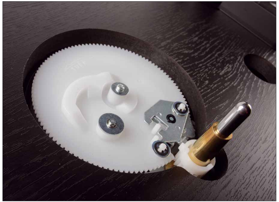
Classic dual gear mechanism and the hardened steel axle in its brass bushing: solid analog technology
