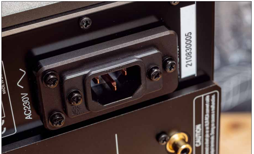
Even the mains input socket is mounted mechanically decoupled
