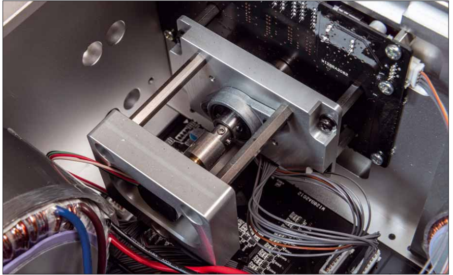
Behind the volume knob is a high-quality rotary encoder
