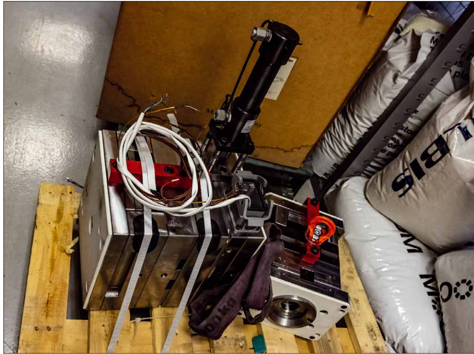
The injection molding tool for the new RCA connector, which is not quite finished yet
