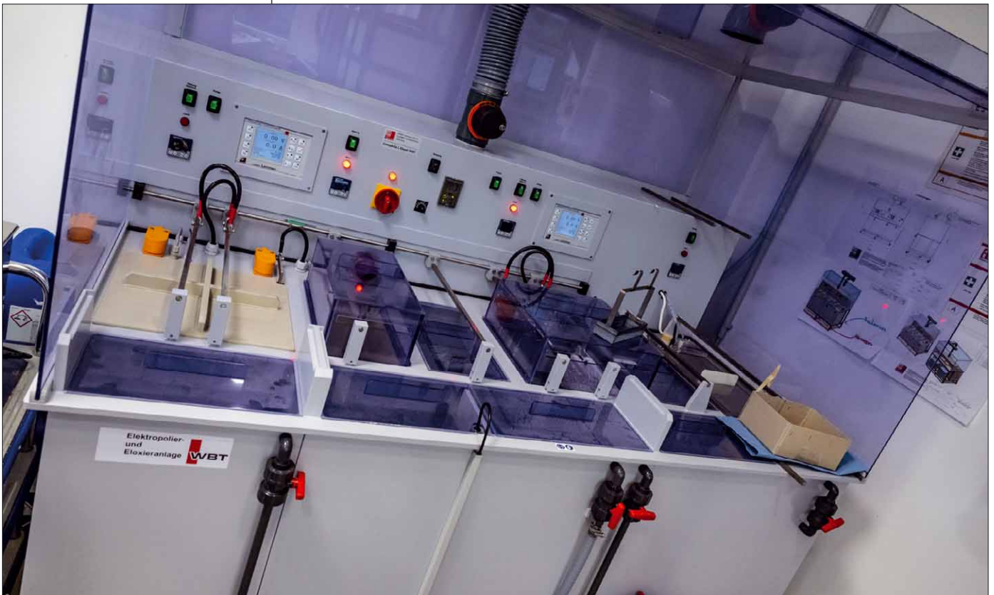
Here, WBT is carrying out tests with anodized aluminum as a contact carrier – it doesn't always have to be copper
