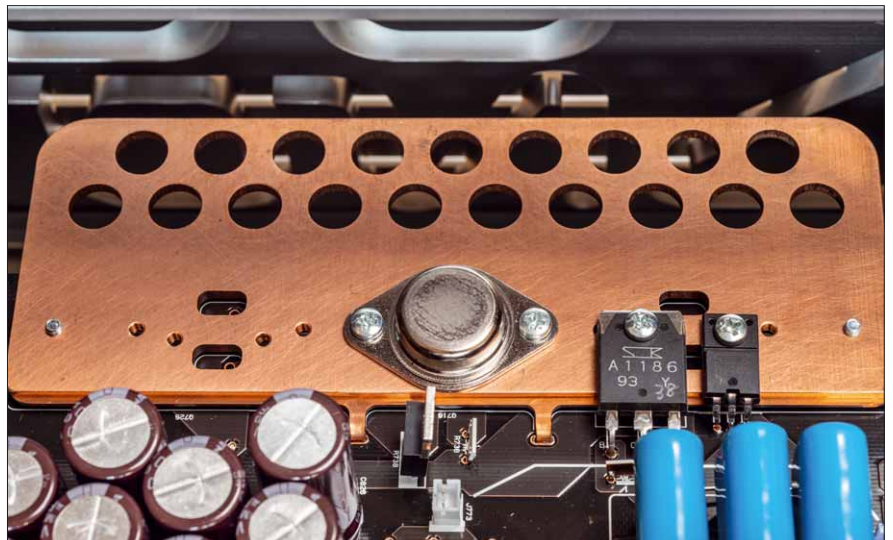
The large metal transistor forms one-half of the actual output stage, the other two next to it are the drivers
