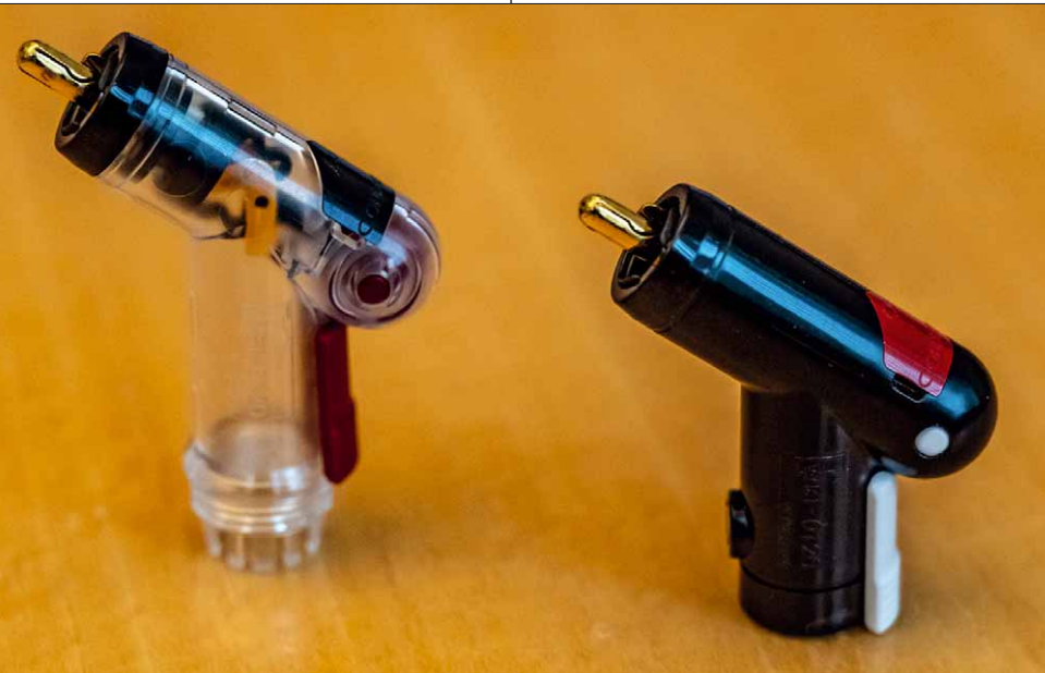
This is the new RCA connector WBT 0120: Series production is expected this year
