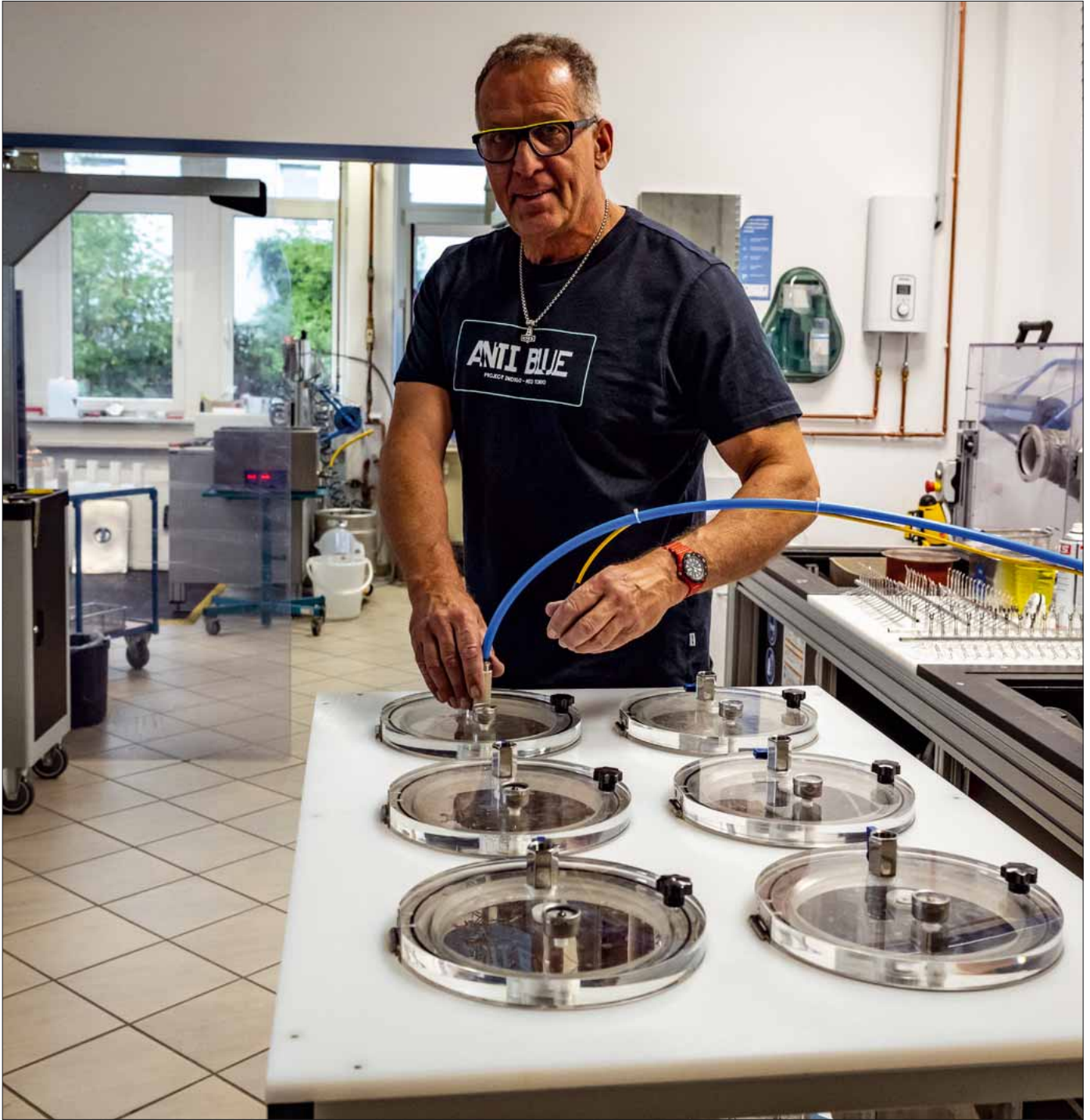
Here, the air is extracted from the new vacuum transport containers
