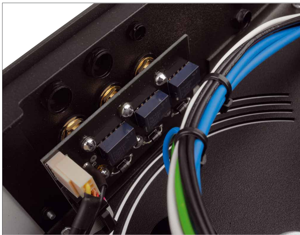
Signals are switched by relay directly at the input sockets
