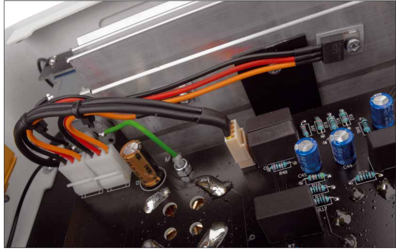
Integrated voltage regulators supply the tube heaters with DC voltage
