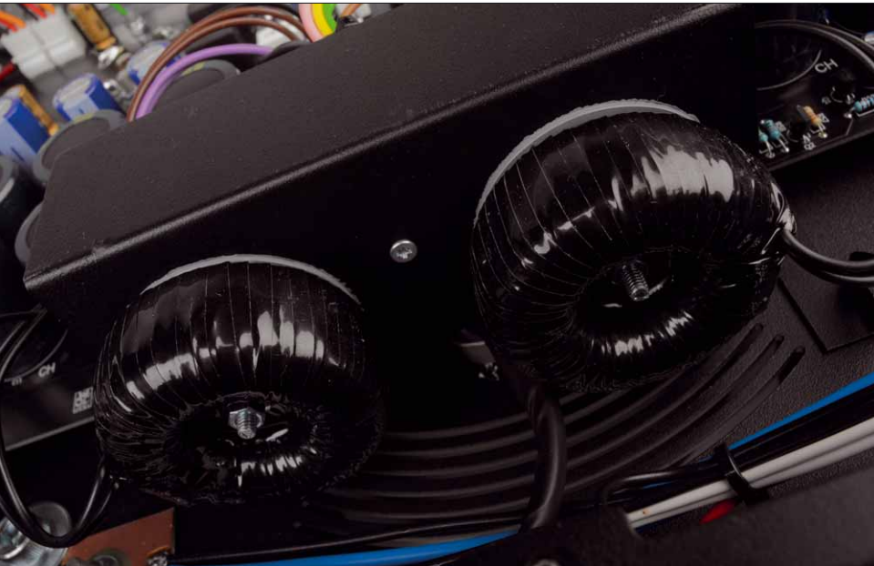
Two toroidal chokes act as screening for the high voltage
