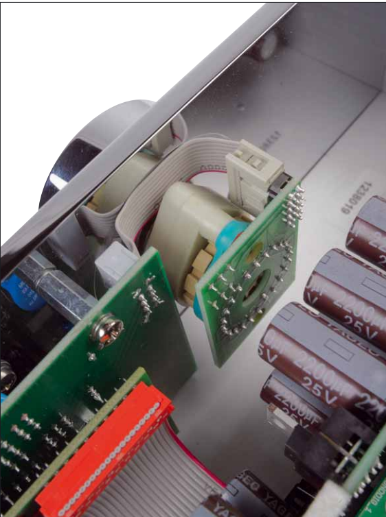
Volume and input selection with fine rotary knobs that only switch control voltages
