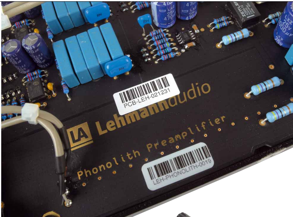
The blue film capacitors are in the equalization
