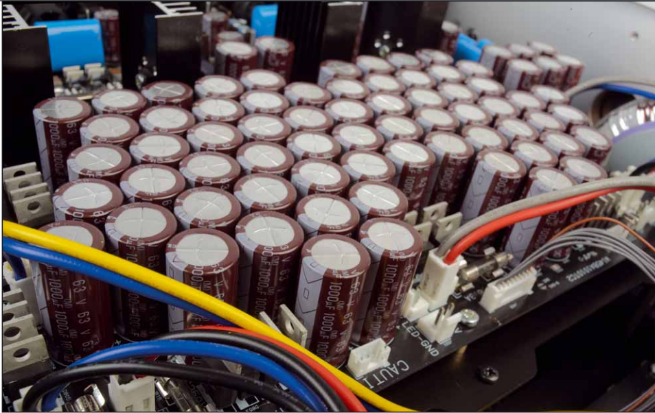
Serious quantities of parallel-connected electrolytic capacitors form the filter capacities of the power supply
