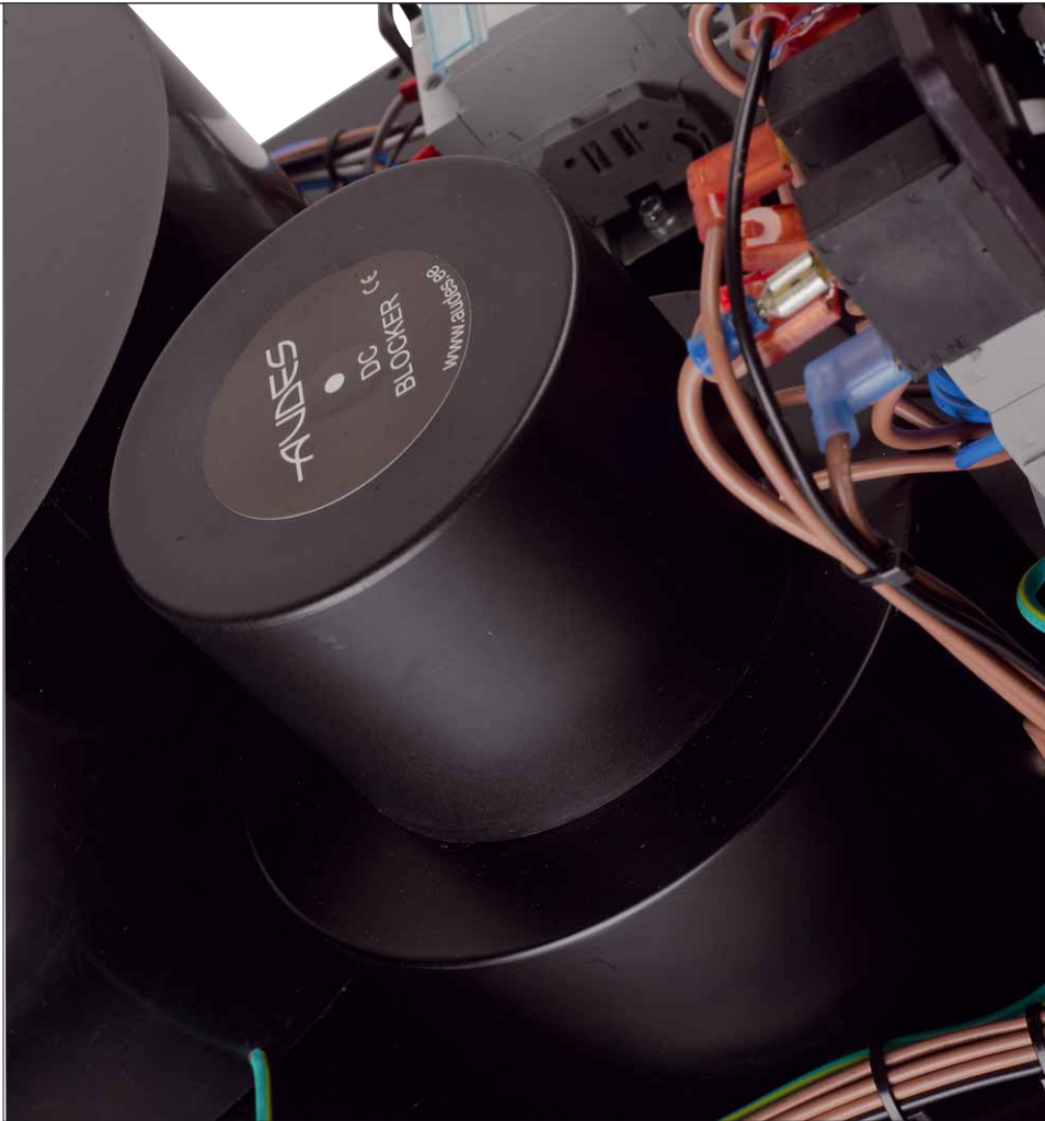
The smallest of the three cylinders inside the device contains the DC blocker
