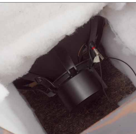
The bass can only be accessed through a flap in the floor. Note the powerful AlNiCo magnet
