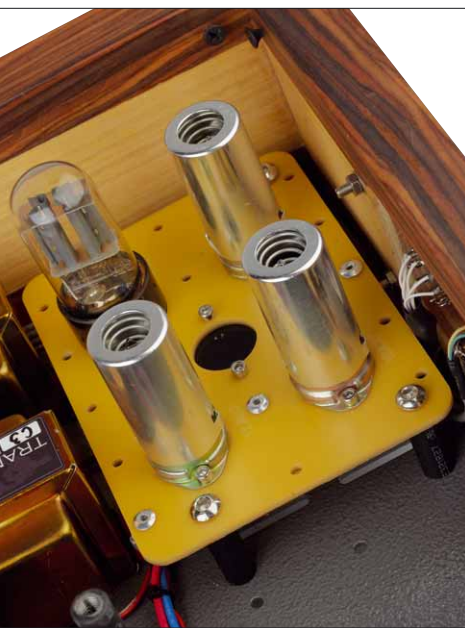
The three Noval tubes do their job protected by shielding cups
