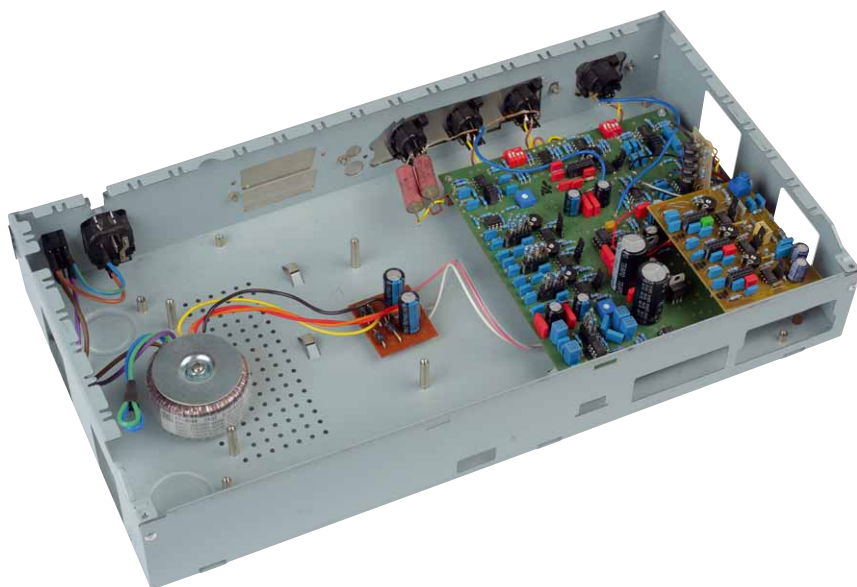
One channel of the still somewhat provisional three-way active crossover
