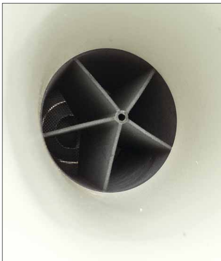
This is the sound guide inside the high-frequency funnel
