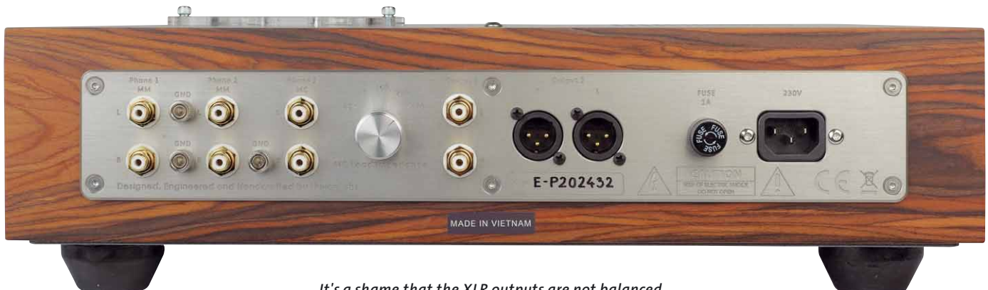
It's a shame that the XLR outputs are not balanced
