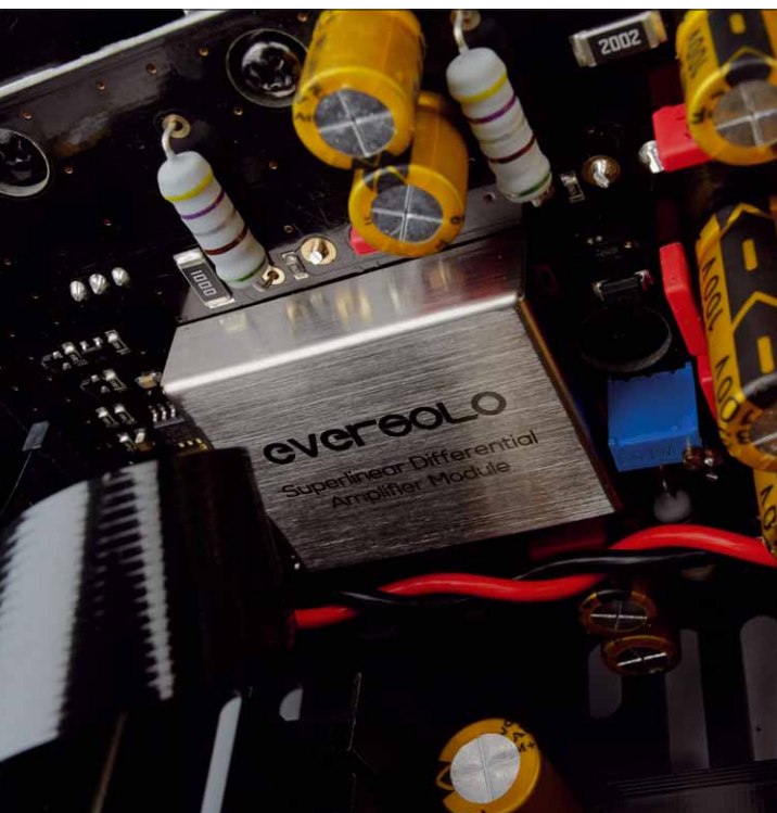
The preamplifier modules are housed in shielded boxes
