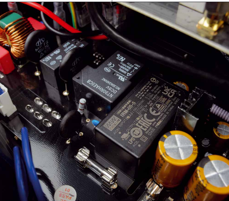
The small switching power supply on the right supplies the circuit components that are active in standby mode
