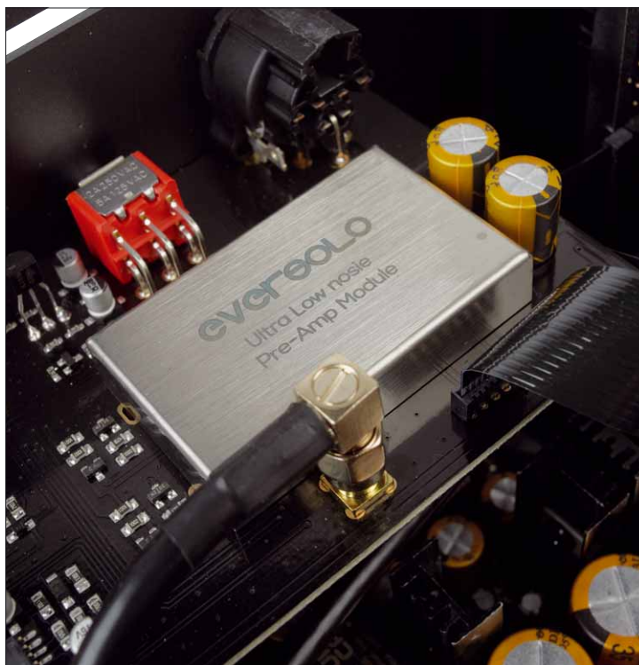
Signal transport via neatly assembled high-frequency cable – something you don't see very often
