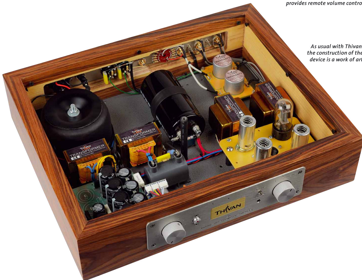
An ALPS motor potentiometer provides remote volume control
