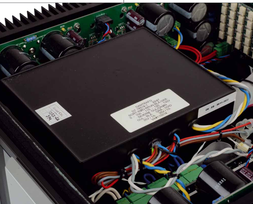
The mains transformer is housed in a separate shielded enclosure.
