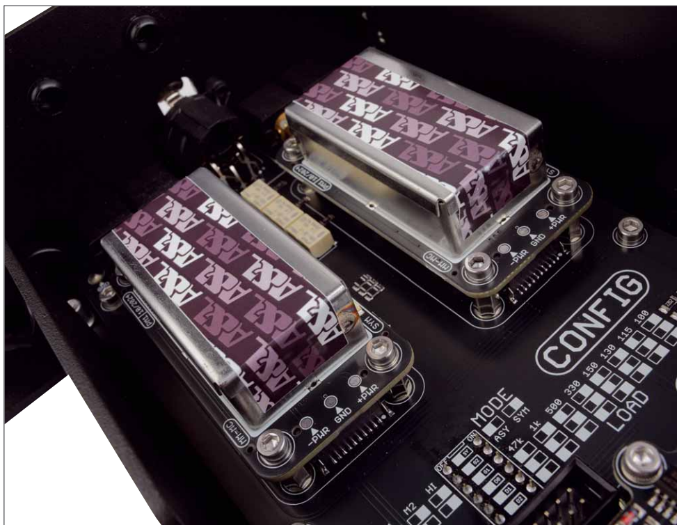
The two phono modules handle all signal processing in the Vinyl Engine
