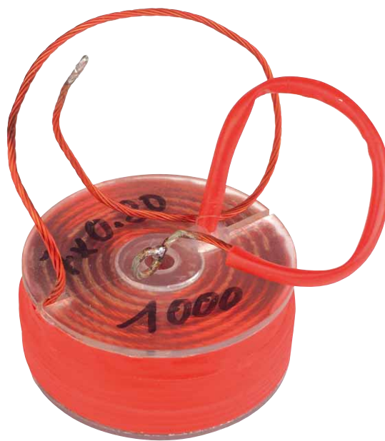
Tritec voice coils made of six twisted individual wires are the material of choice in some parts of the crossover
